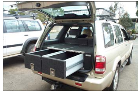
BW900S Twin drawer system fitted to Pre 2005 Nissan Pathfinder with inbuilt fridge slide
