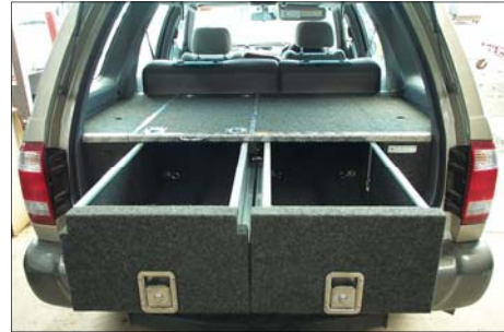
BW900S Twin drawer system fitted to Pre 2005 Nissan Pathfinder with inbuilt fridge slide
